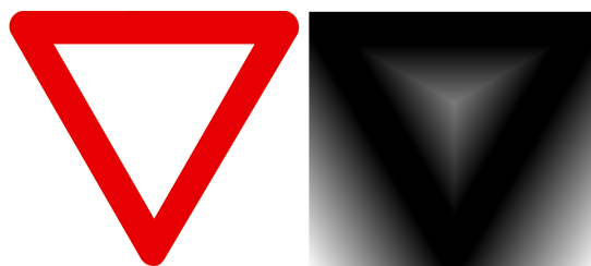
Figure 2.11: Distance Transform. The lighter the pixel, the further it is from an edge.
