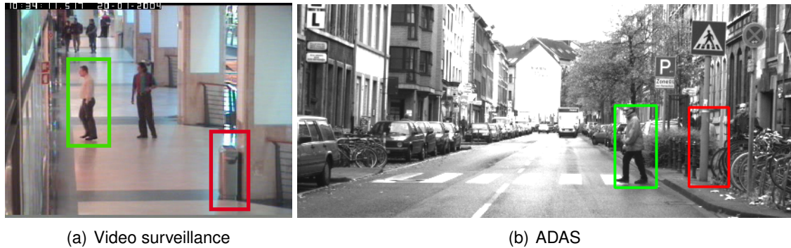
Figure 1.1: We propose two approaches to eliminate false alarms in video surveillance and ADAS systems. Green: validated detection, red: discarded false alarm.
