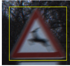
Figure 4.9: Tight bounding box around the traffic sign used for computing the HOG 4 feature
