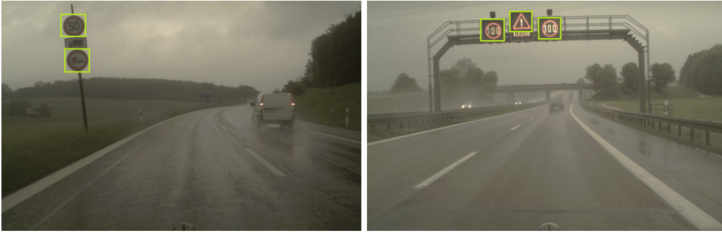
Figure 4.4: Examples of traffic sign detection using HOG/linear SVM. The undirected gradients used in the HOG detector allow for the detection of static and illuminated traffic signs.
