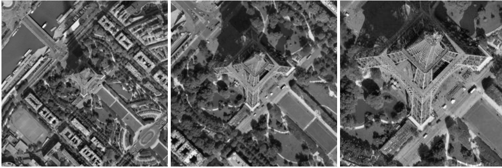
Figure 2.1: Images centered on the same spot with three different resolutions. From left to right: 2m, 1m and 60cm.
