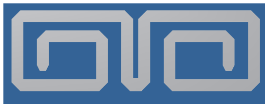
Figure 1.19: Pattern used to make the copper strip. The strips are 3 mm wide and the pattern is 15 mm high. After being cut, the pattern is stuck around a glass tube.
