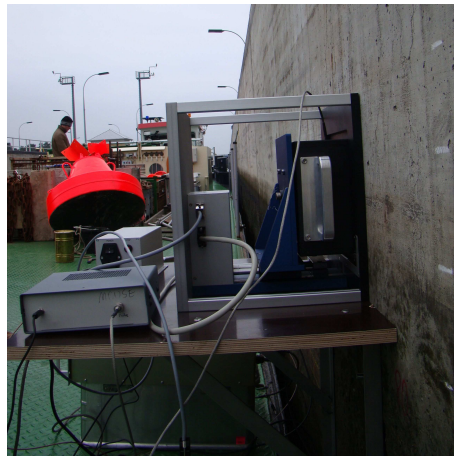
Figure 3.1: Picture of the NMR-MOUSE™ used to scan the lock of Hohenwarthe (Germany).
