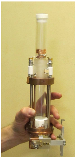
Figure 2.13: Picture of our STRAFI probe. The compatibility with the cylindrical geometry is preserved so the probe can be fixed and the sample move freely inside the glass tube.
