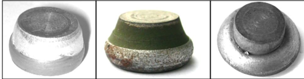
Figure 2.42: Dissimilar metal preforms after hot compression to 50% reduction showing the effect of (a) small difference (Cu–Al), b) intermediate difference (stainless steel–steel) and, (c) large difference (steel–Cu) in flow stress between the base metals. (Domblesky & Kraft, 2007)
