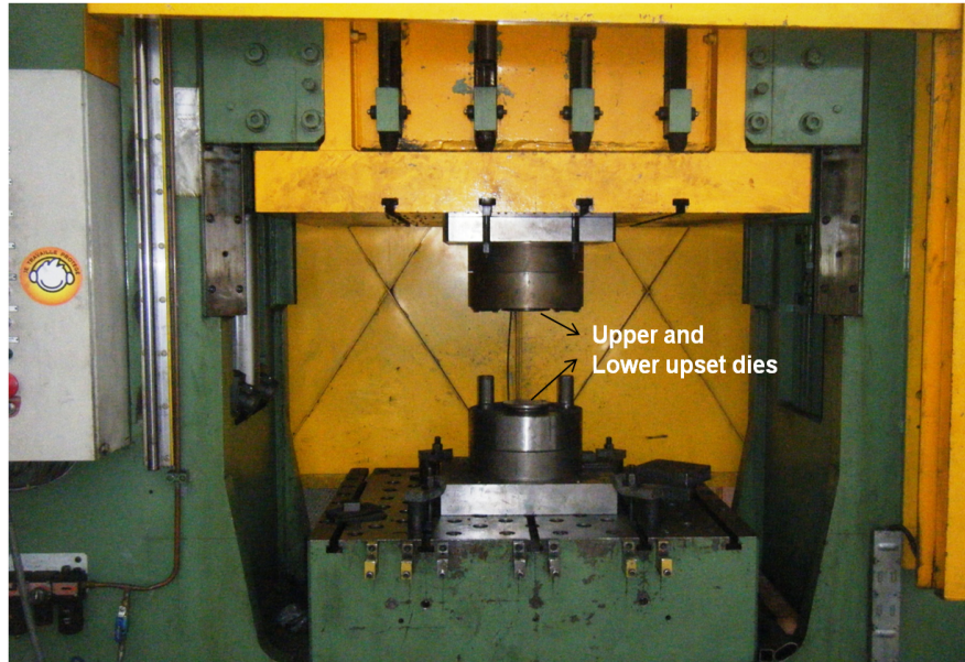
Figure 4.64: Setup for the experimental upsetting test
