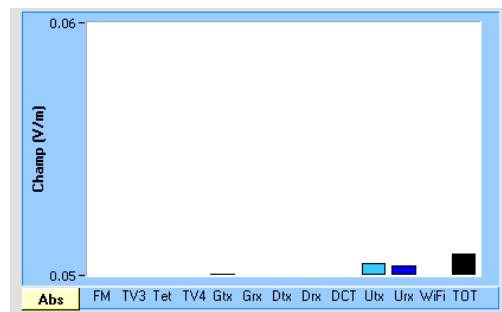
Figure 3.21: Detected frequencies with shielding.
