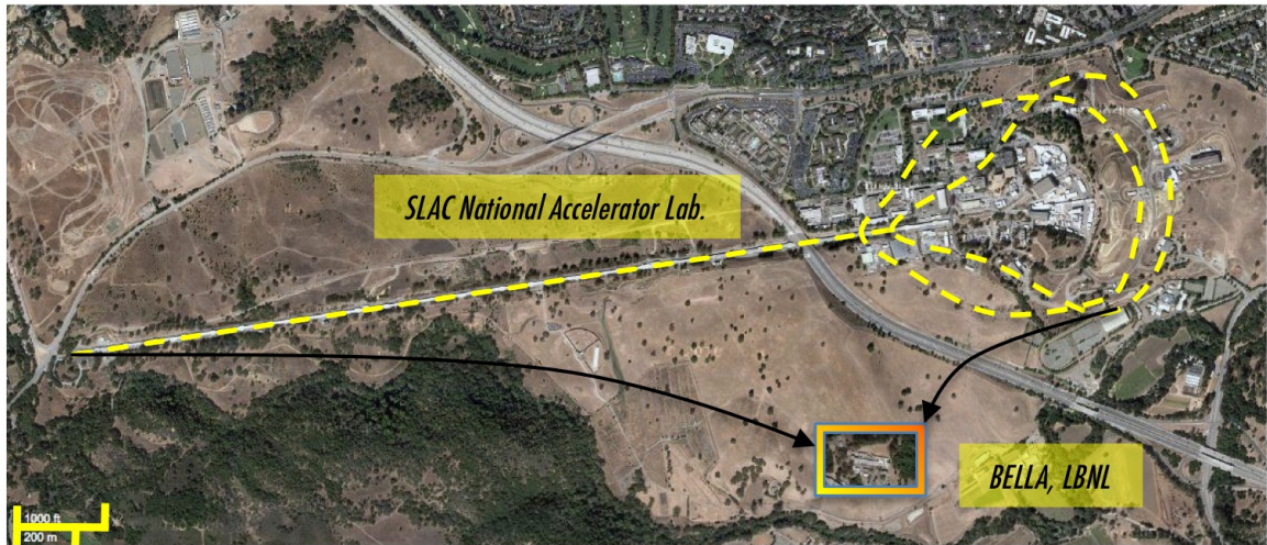
Figure 1.1: An example of conventional linear accelerator facility, the SLAC national accelerator laboratory; and an example, at the same scale, of laser-plasma accelerator, BELLA at the LBNL. ©2010 Google – Imagery ©2010 DigitalGlobe, USDA Farm Service Agency, GeoEye, U.S. Geological Survey
