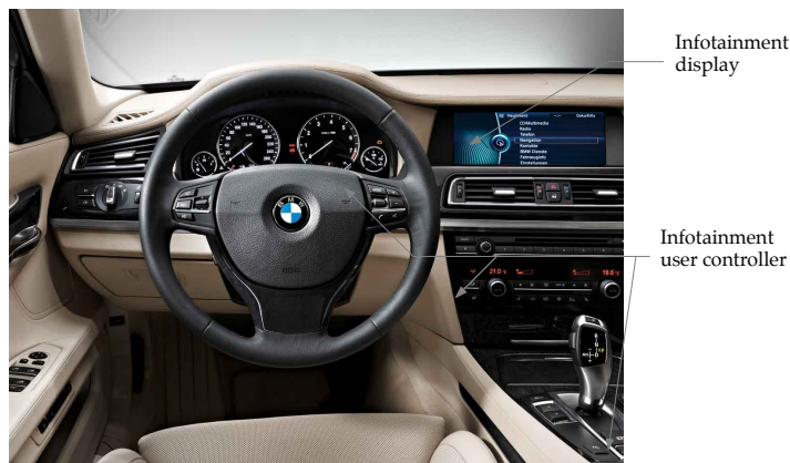
Figure 9: The infotainment controls and display in a vehicle of the premium segment (image BMW)
