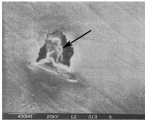
Figure 4.3: SEM micrograph of a typical cavity after a creep elongation of 5% at 650°C under an applied stress of 80 MPa [21].
