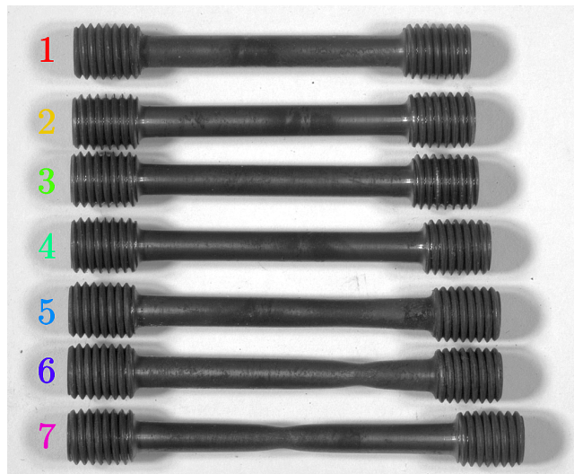
Fig. 2.7. The seven specimens after interrupted tensile tests.
