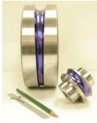
Figure 7. The variable groove on the VMR die (left) requires complex design and manufacturing technology for both dies and mandrel. By contrast, the simple, constant-cross-section HPTR die (right) and similarly simple cams and mandrels allow themselves to conventional manufacturing technologies [Nerino et al. , 2011].
