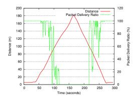
Figure 11.1: UDP range test with 2 cars (distance/PDR)
