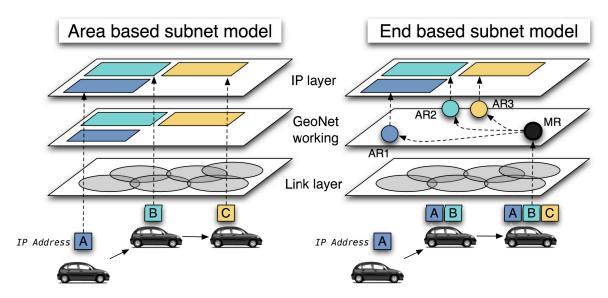
Figure 8.7: Area based link and MR based link
