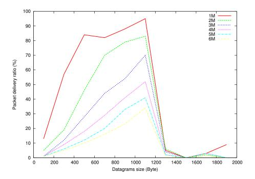
Figure 12.16: Packet delivery ratio between MNN and CN
