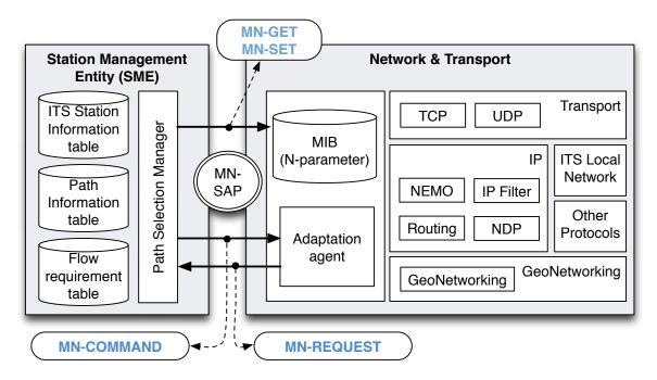
Figure 5.3: Interface Between Management Entity and Network Layer
