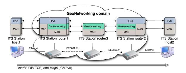
Figure 10.5: Indoor Network configuration
