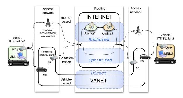
Figure 4.1: Paths between vehicle ITS Station
