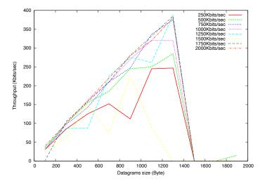
Figure 13.5: UDP throughput in single hop case
