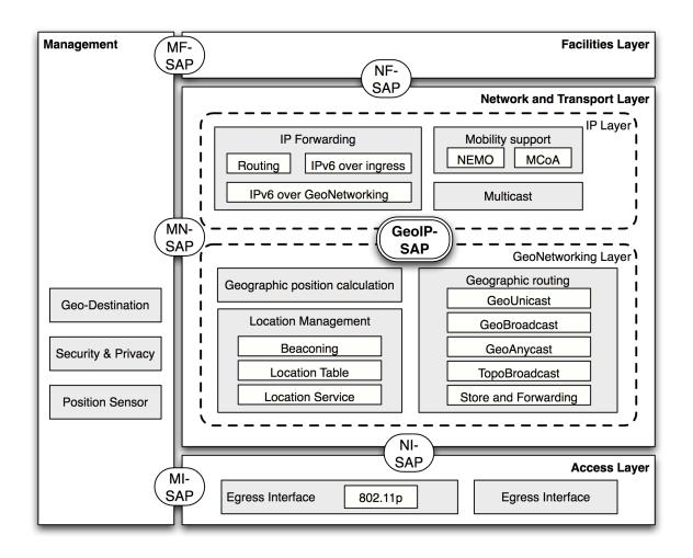
Figure 8.1: GeoNet main functional modules and SAPs
