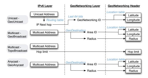
Figure 8.5: SAP for IPv6 over GeoNetworking
