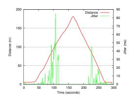
Figure 11.2: UDP range test with 2 cars (distance/jitter)
