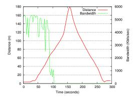
Figure 11.3: TCP range test with 2 cars (distance/bandwidth)
