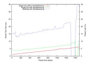
Figure 12.8: Overhead of IPv6 over GeoNetworking
