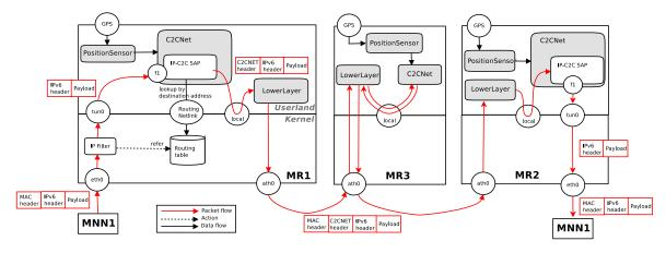
Figure 9.5: Implementation Overview of IPv6 over GeoNetworking
