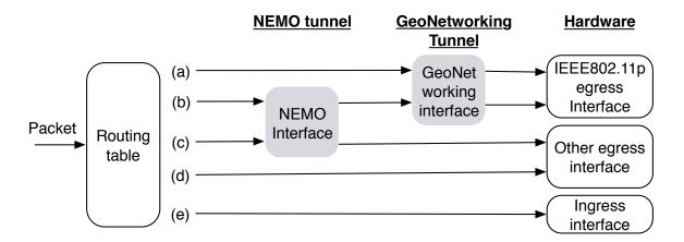
Figure 8.4: Interface management for IPv6 GeoNetworking
