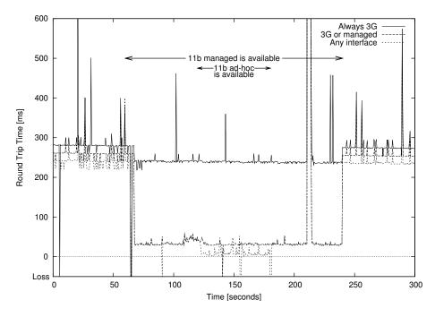
Figure 11.14: Impact of path changes on the RTT, measured using ICMPv6 packets in the absence of background traffic
