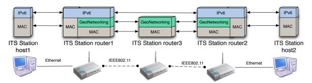
Figure 8.2: GeoUnicast in vehicle-based communications
