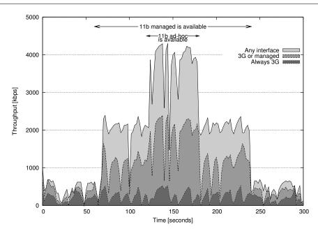
Figure 11.16: Evolution of the throughput of three TCP flows between MNNs using routing policies
