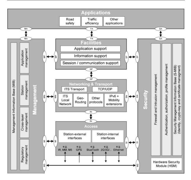
Figure 2.6: ITS station architecture
