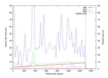
Figure 13.1: ICMPv6 performance in single hop case
