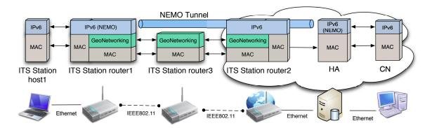
Figure 8.3: GeoUnicast in roadside-based communication
