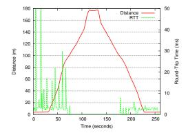
Figure 11.4: Ping range test with 2 cars (distance/RTT)
