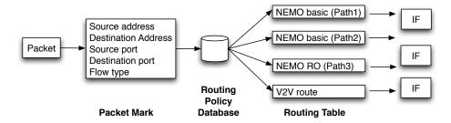
Figure 9.3: Multiple Routing Tables
