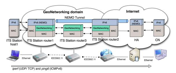
Figure 10.6: Network configuration of the indoor test
