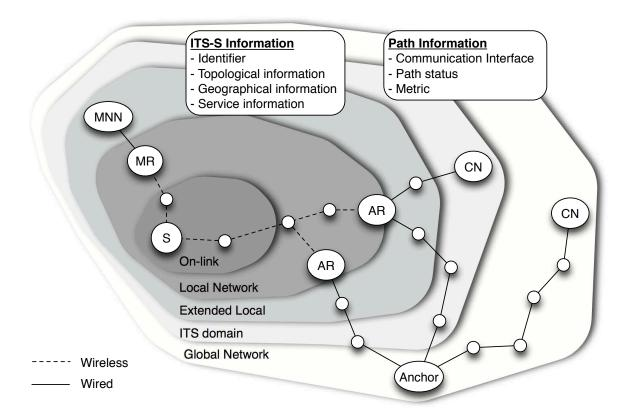
Figure 6.2: Network around vehicle ITS station
