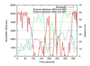
Figure 11.11: TCP highway test with 3 dynamic cars (bandwidth/distance)
