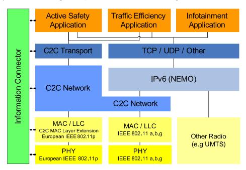
Figure 2.4: C2C-CC and GeoNet Architecture
