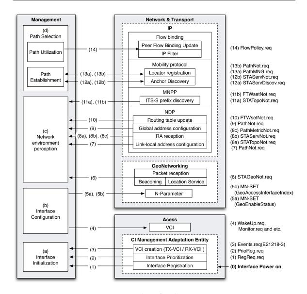
Figure 7.4: Procedure of Path Management
