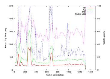
Figure 13.2: ICMPv6 performance in multi-hop case
