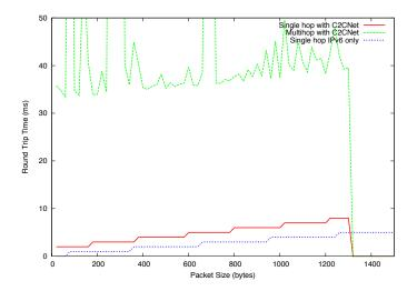
Figure 13.3: Overhead between GeoNetworking and IPv6
