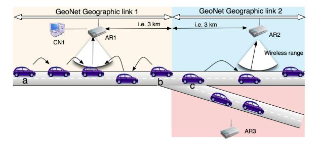
Figure 8.6: Area-based subnet model in GeoNet Project
