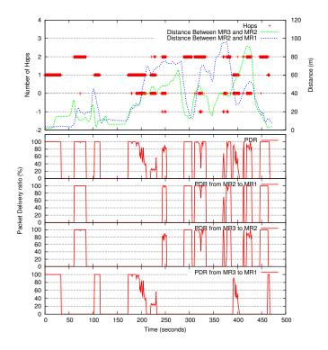
Figure 11.10: UDP highway test with 3 cars
