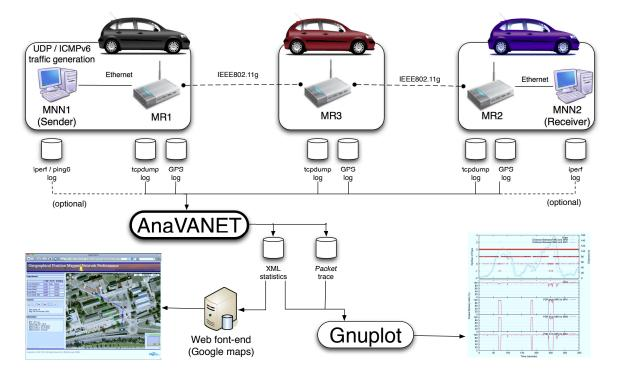
Figure 10.8: AnaVANET: Overview of packet processing and analysis
