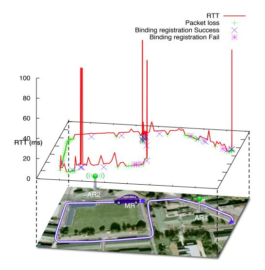
Figure 13.6: RTT, Packet Loss and Mobility Signaling of ICMP evaluation in handover scenario
