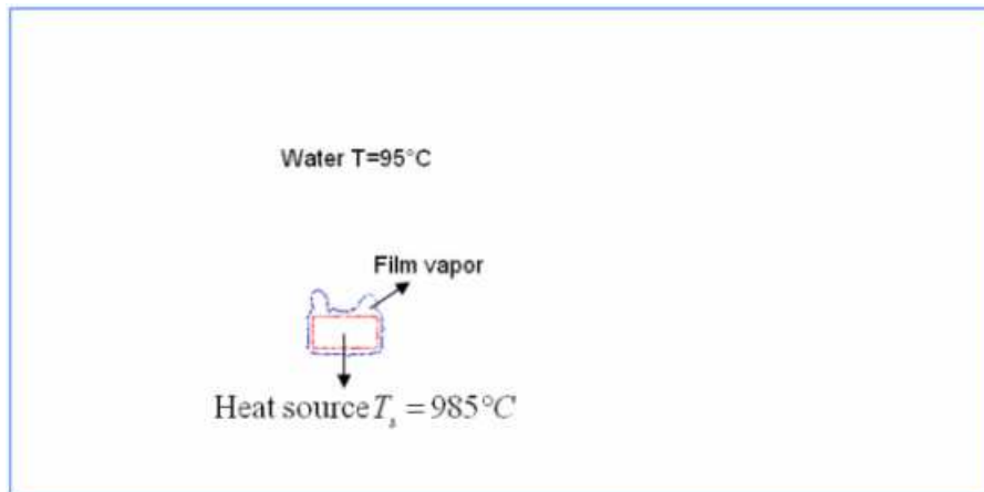
Figure 5.6: Two dimensional film boiling interface profile computed on a large scale grid
