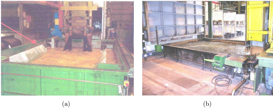
Figure 1.6: Different baths (Snecma): (a) Polymer tank 18 m 3 , agitated by 6 pumps, (b) Water tank 35 m 3 , agitated by 2 pumps
