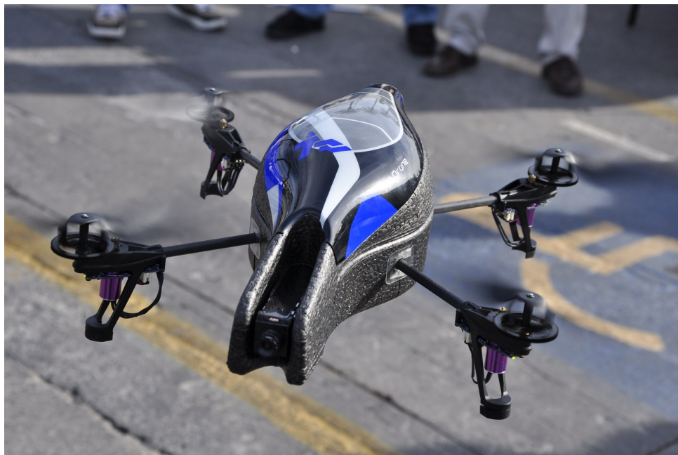
Figure 8.1: Parrot AR.Drone, with its outdoor hull.
