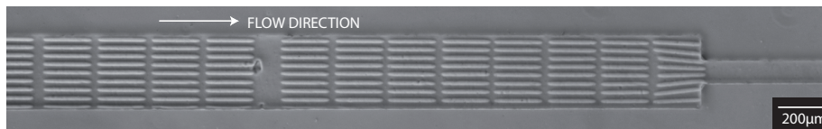
Figure 7.2: Top view of the microchannel in the second flow configuration at the initial state. The fibers are fabricated by groups of eight, all parallel to the flow direction.
