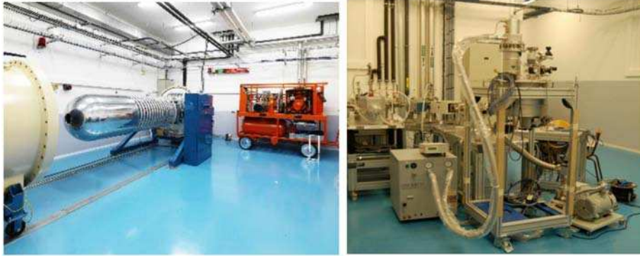
Figure 9.3 A photograph of the SIRIUS Accelerator of the LSI. On the right-hand side the cryostat used for the irradiation at low temperature is presented.
