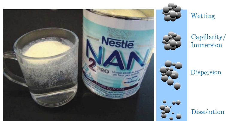
Figure 1.1: Beverage reconstitution process - (Picture) Reconstitution of a dehydrated dairy powder. (Scheme) Reconstitution process is often decoupled into 4 steps.
