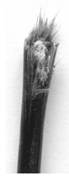
(b) Creep rupture in torsion-bending
