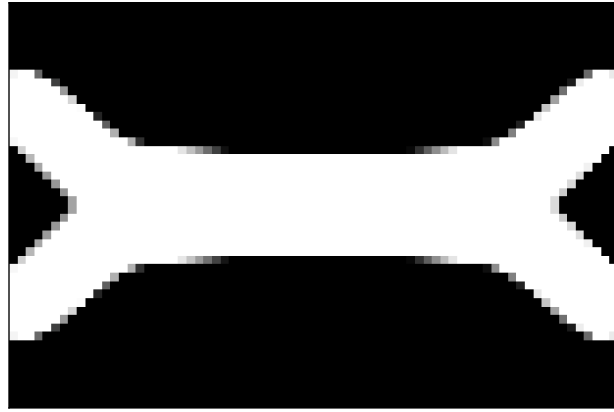
(c) Result of topology optimization for L = 1.5\ell ( 72 \times 48 design parameter grid).
