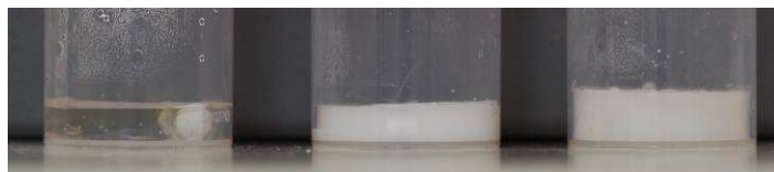
Figure 14: Pictures of hybrid hydrogels synthesized at pH 5. Left: SP0, centre: SP2, right: SP5.
