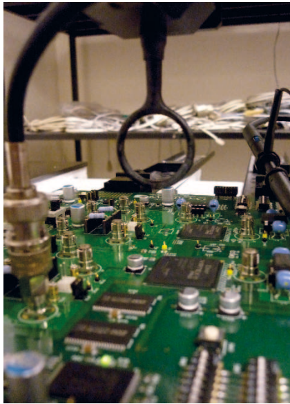
Figure 6.10: EM loop on the SASEBO Board during an RSA computation.
