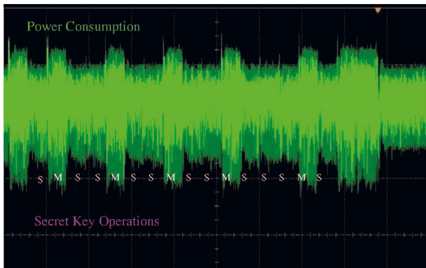
Figure 1.3: RSA power supply consumption on a FPGA.
