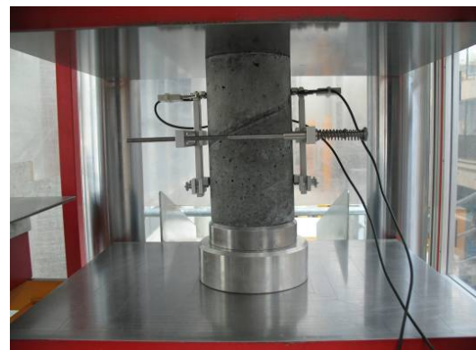
Figure 3-11: HPFRC cylinders after the failure, formulations B2 to B5 and E-modulus test
