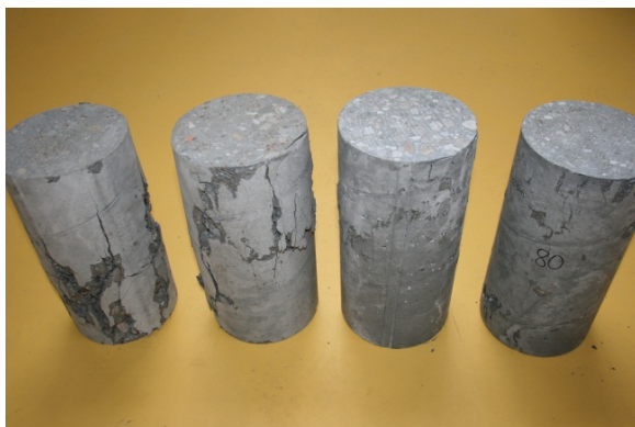
Figure 3-11: HPFRC cylinders after the failure, formulations B2 to B5 and E-modulus test
