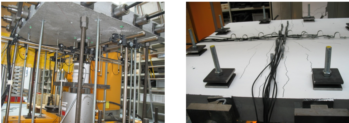
Figure 5-12: Views of the deflections and top strains measurements
