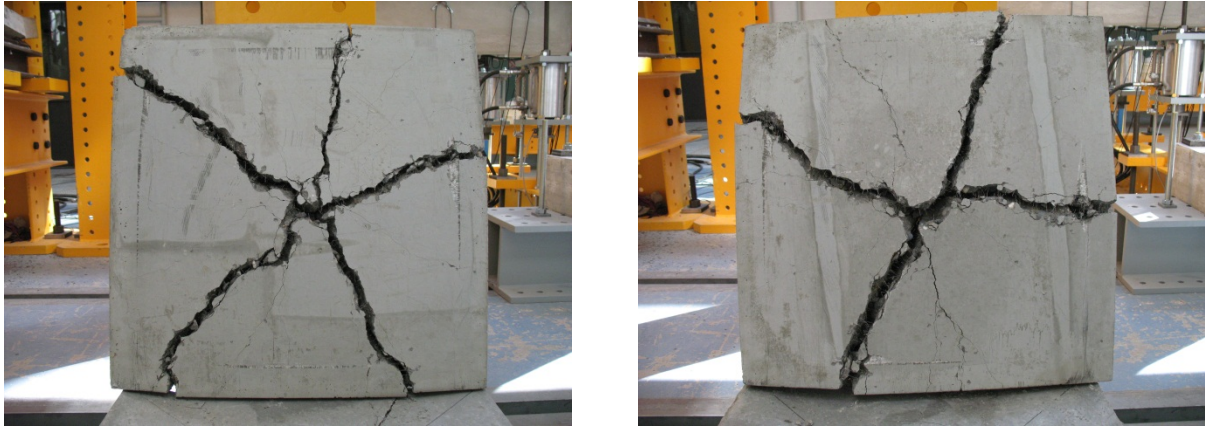
Figure 3-21: Typical cracking pattern of bending test on square slabs, n=5 and n=4
