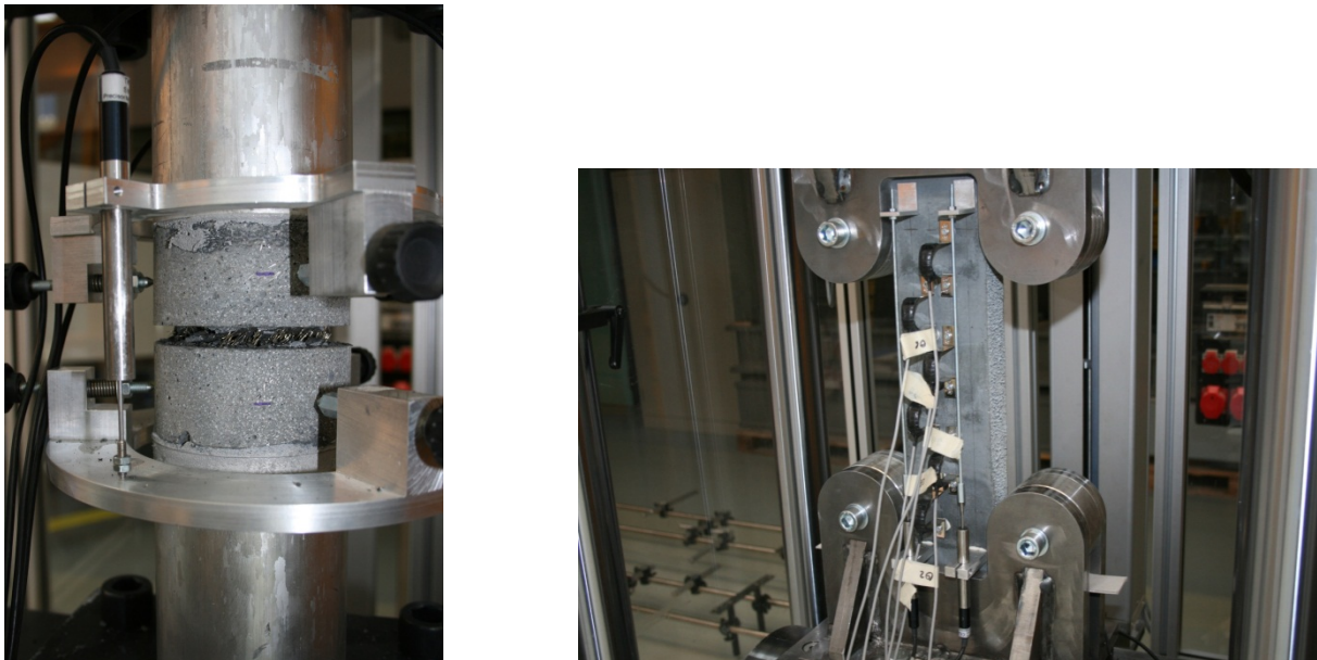
Figure 2-14: Uniaxial tensile test performed on notched core and “dog bone” element
