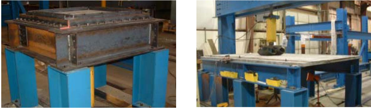
Figure 2-119: Views of loading setup of small and large UHPFRC slabs
