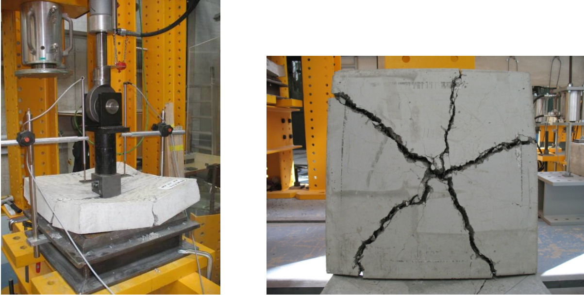
Figure 2-17: Load test on square slabs according to SIA162/6 [SIA1999] and typical cracking pattern
