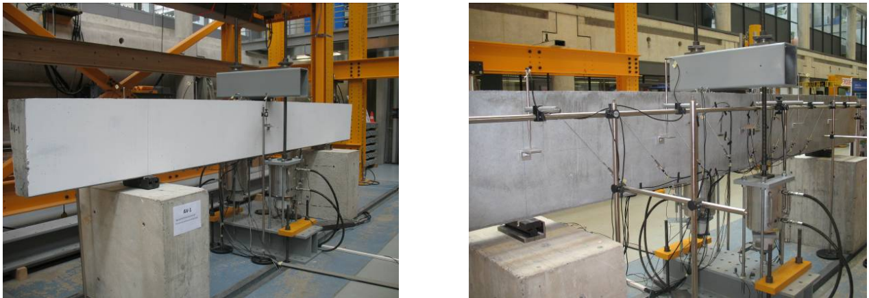
Figure 4-23: Views of the shear beams setup and measurement arrangement
