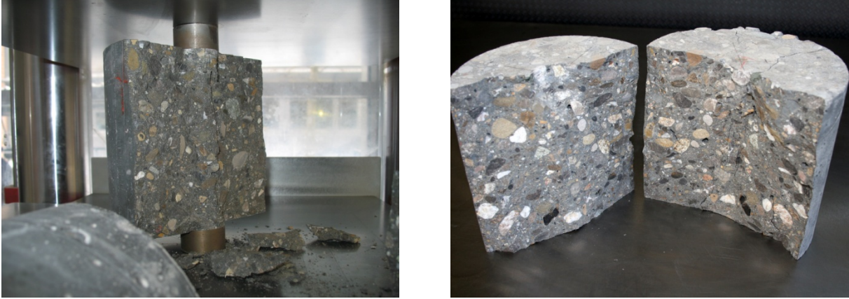
Figure 3-12: Double punching test on HPC cylinders
