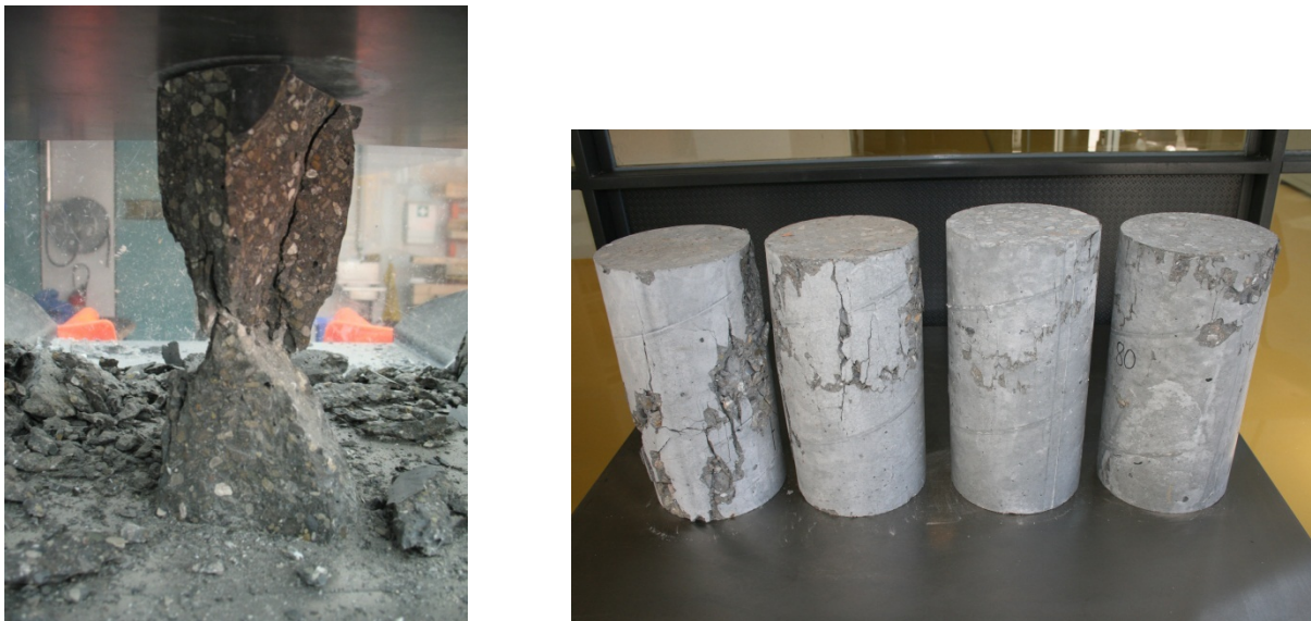
Figure 2-7: Failure of HPC compared to HPFRC
