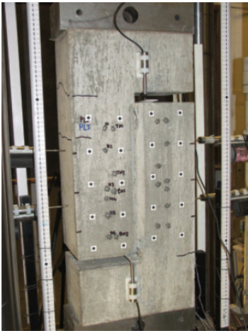
Figure 2-37: Push-off test arrangement [NAG2007]
