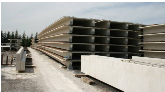
Figure 4-2: Double-tee beams for the construction of an industrial floor
