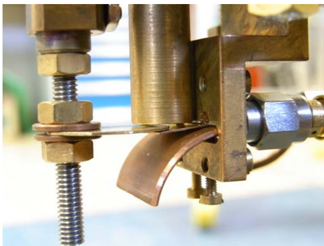
Figure 10.1: Bending setup for sample JT6 fabricated on a bronze substrate. We have used a curved shim made out of copper, to obtain a more distributed bending.
