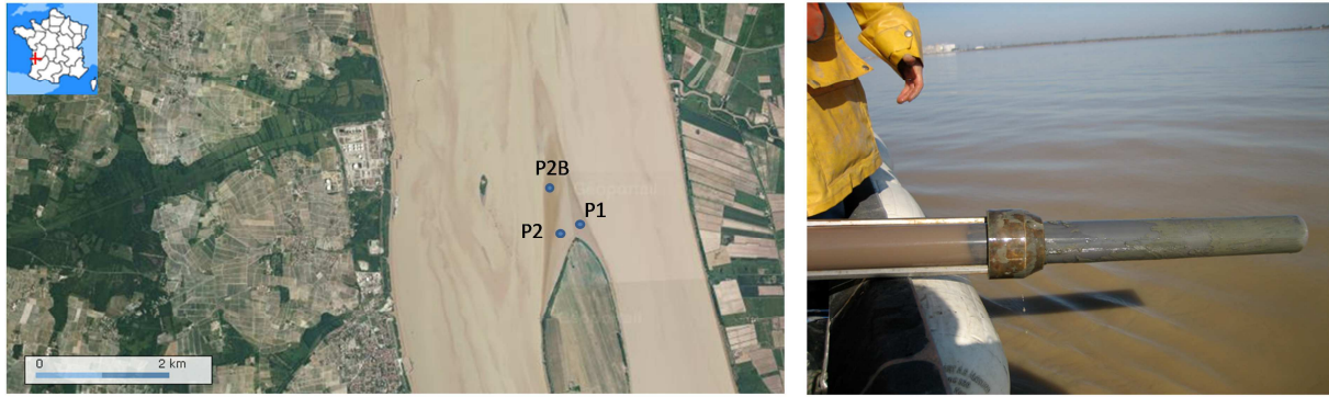
FIGURE 1.18- Location of sediment core sampling points (left). P2B sediment core (right).
