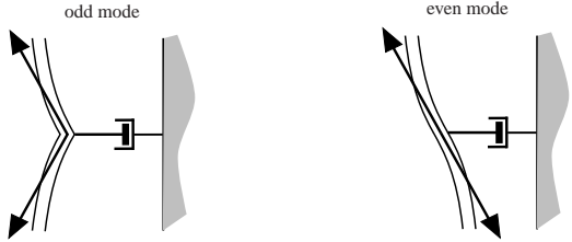
FIGURE 4. LOCAL MECHANISM OF FORCING OF A HARVESTER BY STATIONARY MODES. LEFT : ODD MODES, HIGH EFFICIENCY / RIGHT : EVEN MODES, LOW EFFICIENCY.
