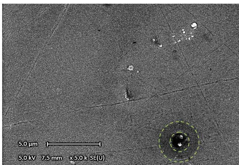
Fig. 19 – SEM image of a methylated a-Si:H electrode after the first electrochemical cycle.
