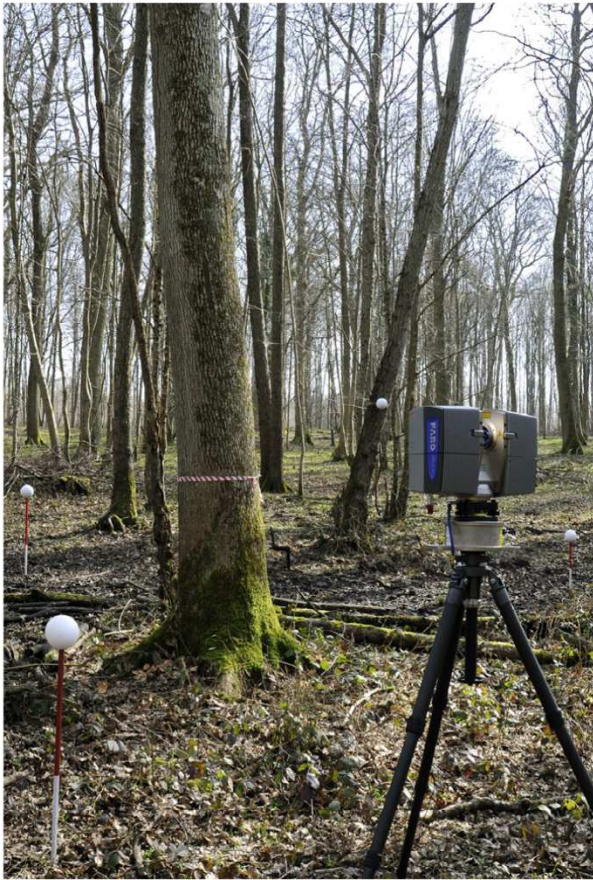
Fig. 1. Field scanning set-up. A FARO Photon 120 scanner mounted on a tripod was used to scan each tree from three or four different positions to obtain a complete description of the woody structure of the tree.
