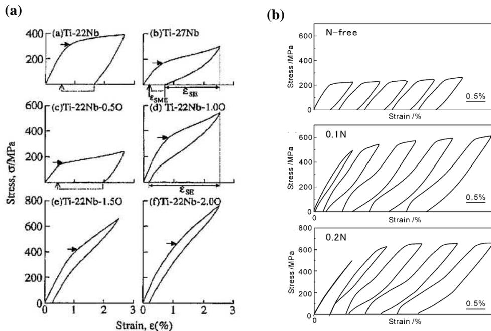
Figure I-20. Courbes de traction de (a) Ti-22Nb-(0,5-2)O (at.%) (Kim et al. 2005b) et (b) Ti-10V-2Fe-3Al (Furuhara et al. 2006).
