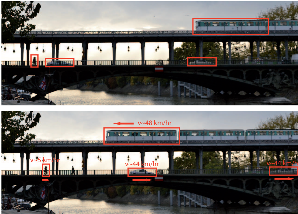
Figure 3.9: The idea behind particle tracking velocimetry.
