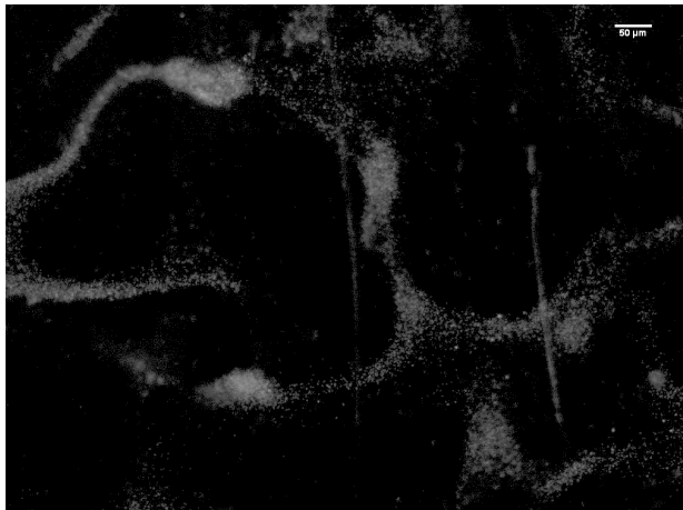
Figure 6.1 Acoustic streaming patterns at the levitation plane for 883nm particles in continuous mode. Scale bar = 50\mu\text{m} , magnification 20X.
