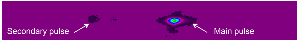
Figure 5.12.: The intensity autocorrelation evidencing the existence of a main and a secondary pulse.
