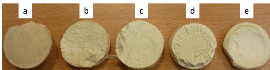
Figure V. 15 : Dried cellulose-CA hybrid monoliths coagulated in ethanol made from mixtures with 10% total polymer concentration: cellulose:CA = 80:20 (a), 60:40 (b), 40:60 (c) and 20: 80 (d), 0:100 (e).
