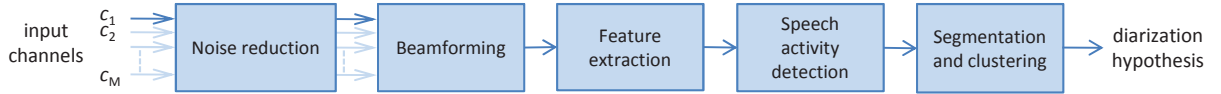
Figure 2.2: An overview of a typical speaker diarization system with one or multiple input channels.
