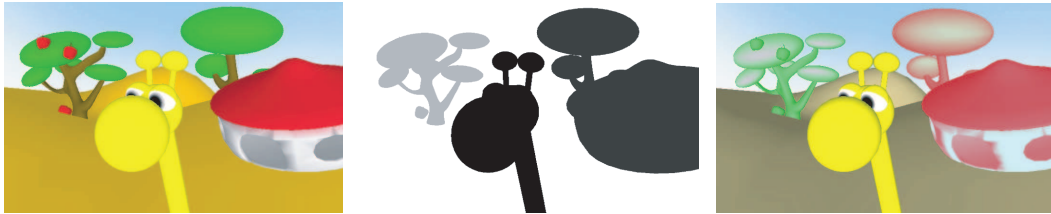
Figure 2.6: 3d Dynamic Grouping for Guided Stylization. Starting from a 3d scene (left), a number of representative samples is clustered in feature space and a « level of abstraction » map (middle) is generated from the clustering and given features. This map is then used to guide the abstraction and stylization of the scene (right). Images taken from [Bez+08].
