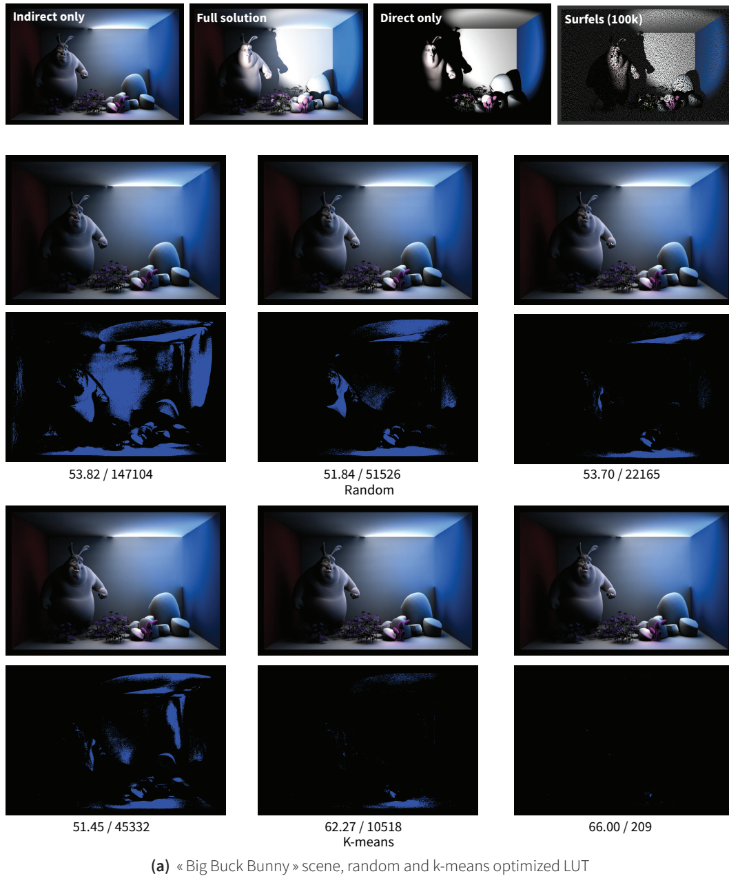
Figure 6.8: Visual comparison (indirect contribution only) between ground truth (top left) and our quantization, using 100 (top middle left), 1000 (top middle right) and 10 000 clusters (top right). The error images (bottom) are the perceptual differences in the Lab color space [Yee04], depicted in black (no visible difference) and blue (visible difference). For numerical comparison, we give the PSNR for RGB images and the number of Perceptually Different Pixels [Yee04] (PDP) below each error image (<PSNR>/<PDP>). The full rendering is displayed on the bottom left. (Figure continued on the next pages.)
