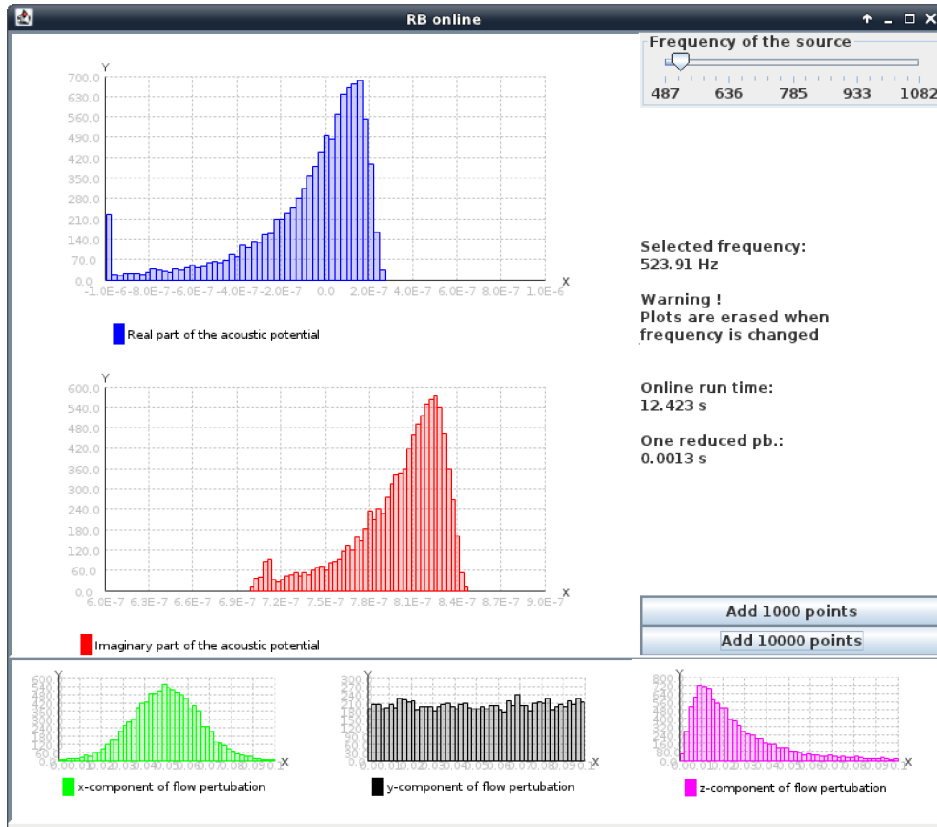
Fig. 7.4. Java applet for the online stage of the reduced basis method for test case 2. Top panel: histograms of the real part and imaginary part of the quantity of interest. Bottom panel: histograms of the three components of the perturbation of the flow
