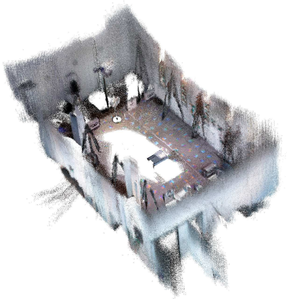
Figure 10.13: Entire view of the reconstructed cartography, computed using filtered position and depth measurements. The reconstructed point cloud is very accurate, since relative errors on direct physical measurements do not exceed 1%. The overall geometry of the reconstructed scene is also very convincing: walls are flat and objects are not duplicated.
