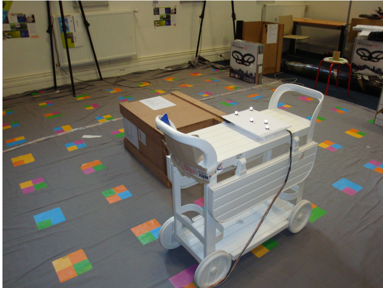
Figure 10.3: The trolley used to ensure that our system is only submitted to pure lateral translation.
