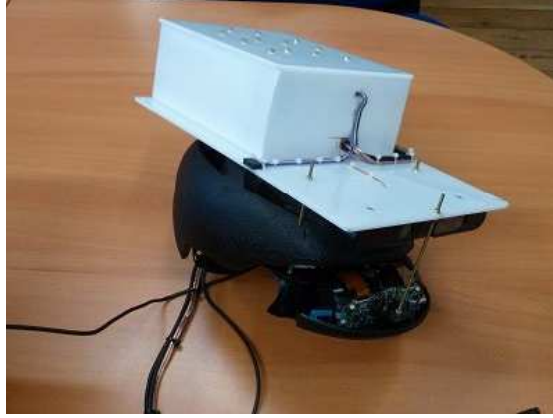
Figure 9.3: Implementation of the augmented reality system, which is intended to be worn on the head: the RGBD sensor and augmented reality glasses are fixed respectively on top and in front of the eyes, to acquire real images and project the augmented images. The magneto-inertial sensors lie on top of the head: all components are linked to an external master system.
