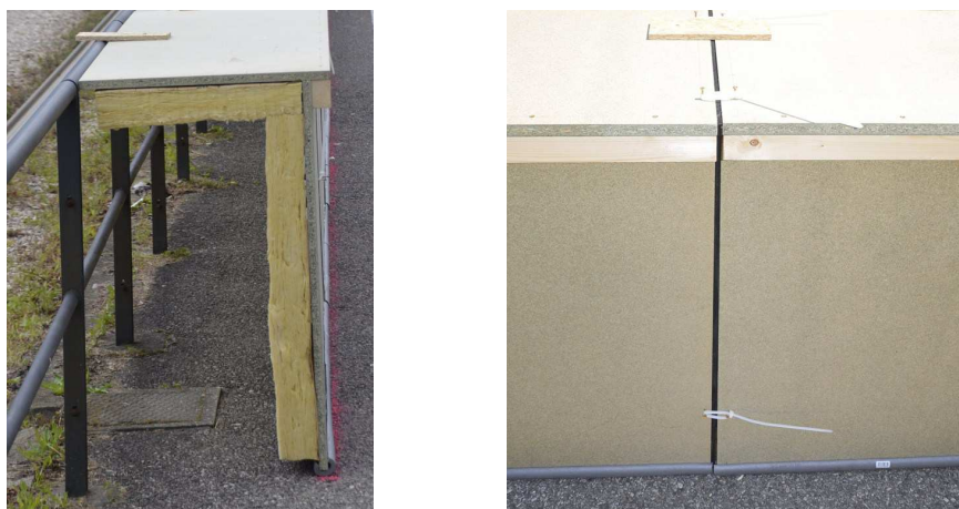
Figure 8.4: Views of the low-height barrier prototype. Left: cross section. Right: joint system between elements.
