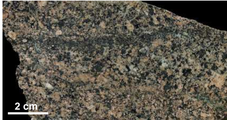
Figure 18 - Granodiorite from Chwalisław Kopciowa mountain showing bands and additional pink feldspars. Dark band seems to be constituted of mafic minerals such as amphiboles and biotites.
