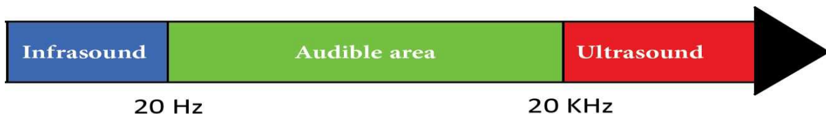
Figure 2.1: Approximate frequency ranges corresponding to ultrasound
