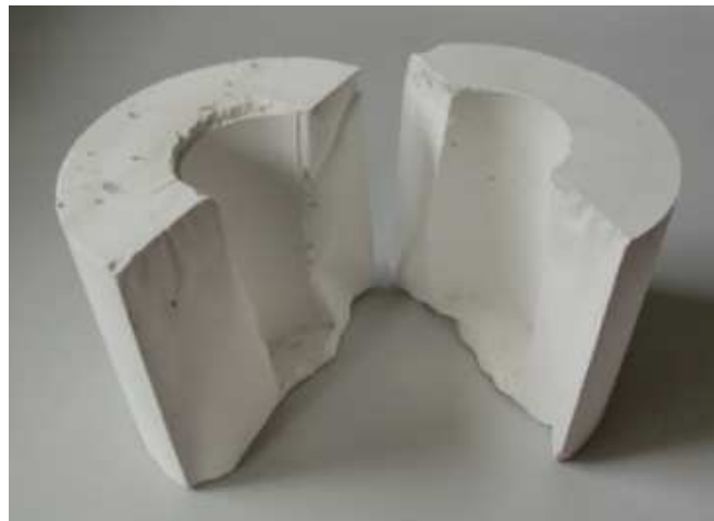
Figure 12.3: Plaster mould used for glass sintering.
