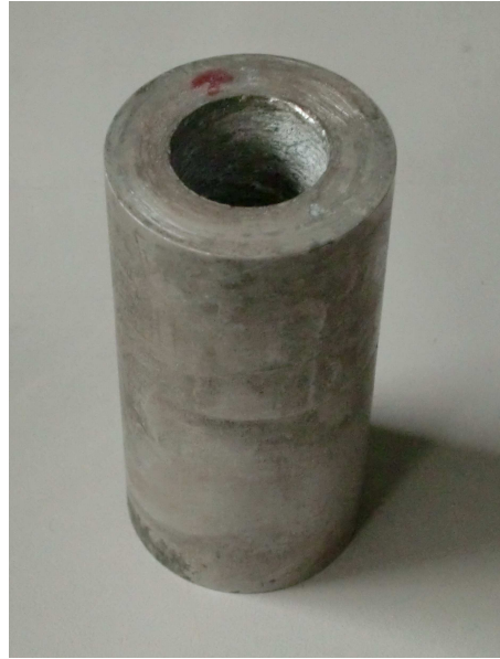
Figure 11.12: Steel tube for dead volume measurement.
