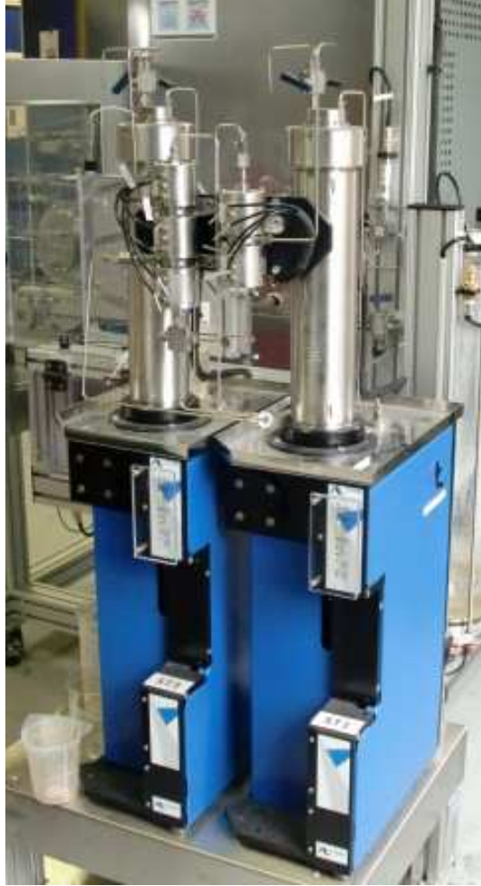
Figure 11.8: STIGMA1000 pump (here ST1 and ST3).
