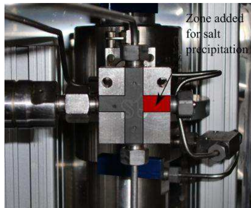
Figure 14.1: Modification of the T junction for salt precipitation.
