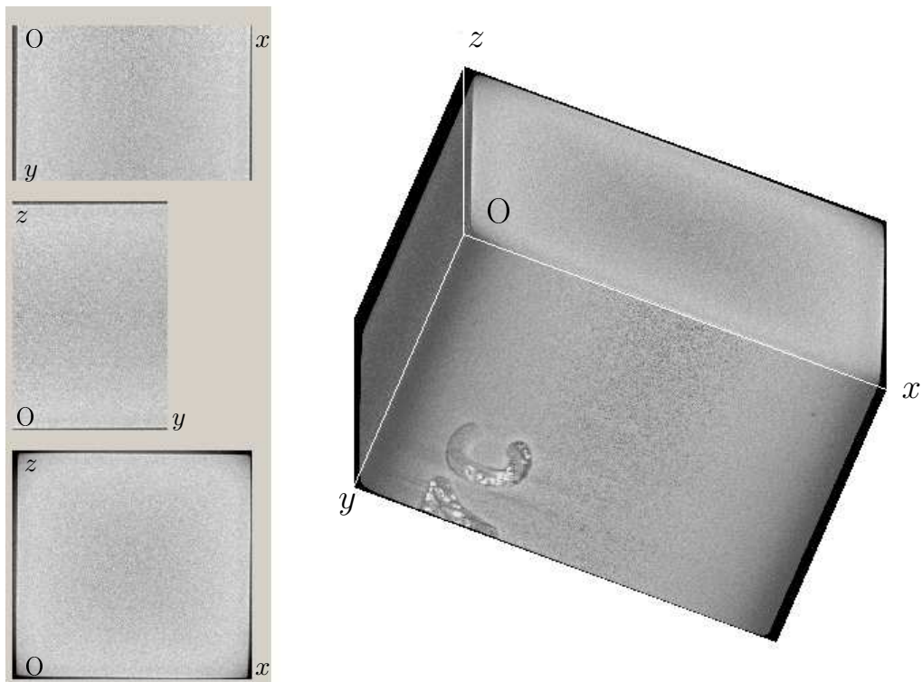
Figure 2.9: Tridimensional raw image of sample T2 (Ti-alloy) obtained using X-ray microtomography, and 2D slices along each spatial direction.
