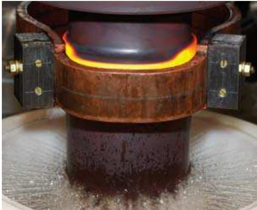
Figure I.4: Spray cooling of induction heated workpiece (Image provided courtesy of EFD)
