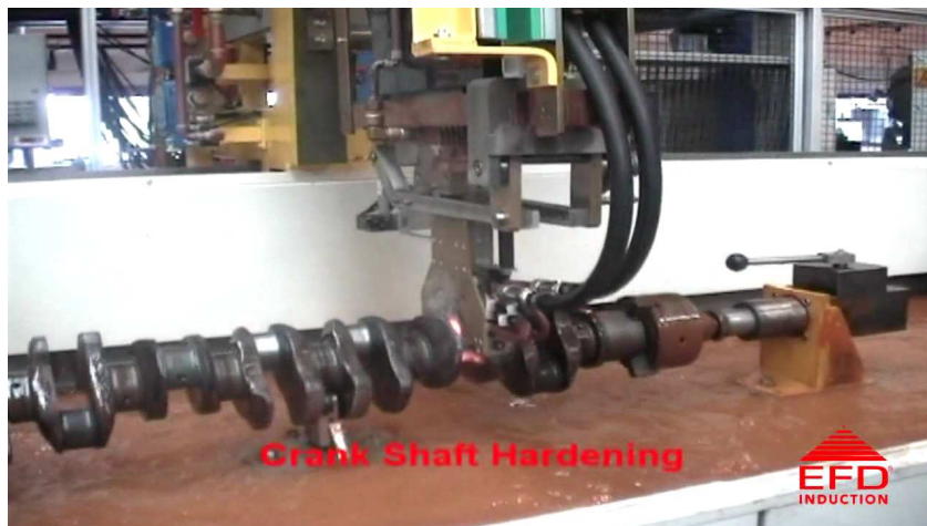
Figure IV.1: Induction heating of a crankshaft (Image provided courtesy of EFD)
