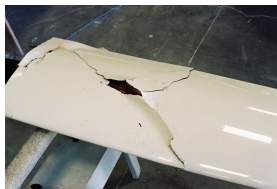
Figure: Buckled wing
