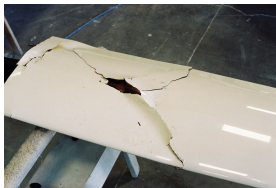
Figure: Buckled wing
