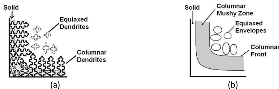
Fig. II-5 Schematic illustration of (a): dendritic growth and (b): mushy zone tracking representation [McF09].
