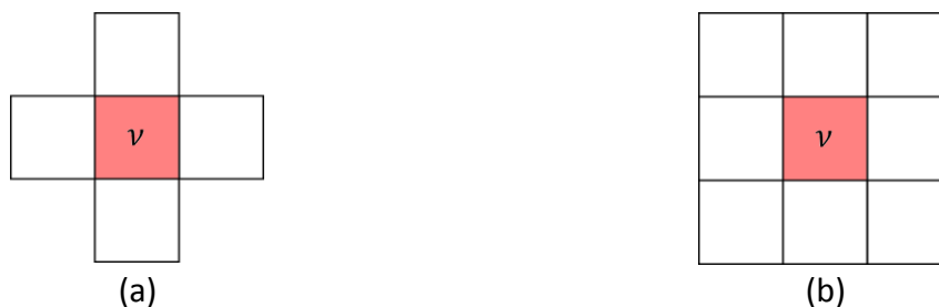
Fig. II-11 Schematic illustration in 2D for (a): the Von Neumann neighborhood, and (b): the Moore neighborhood. In both case, the cell \nu itself is shaded by red color [Mit98]
