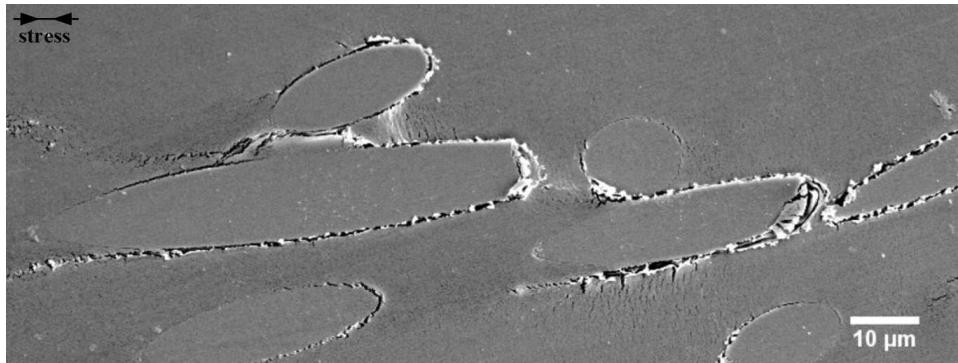
FIGURE 4.30: Damage mechanism in compressive zone of RH = 50%, longitudinal specimen at 99% \sigma_f .
