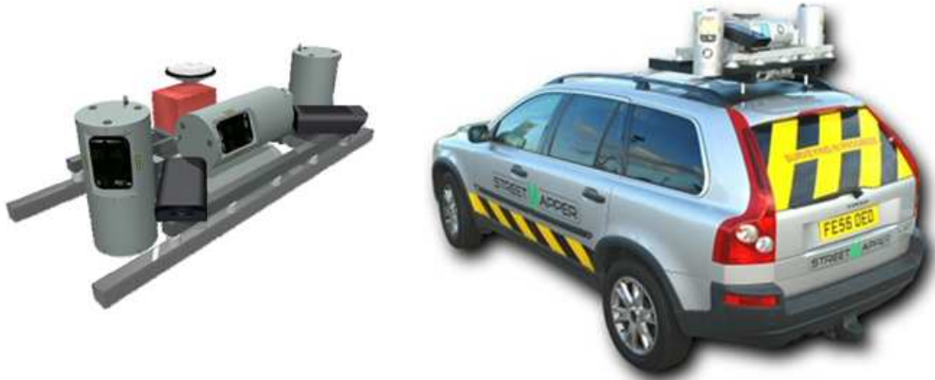
Figure 2-26 : StreetMapper, système de 3DLM (source [web 3DLM])
