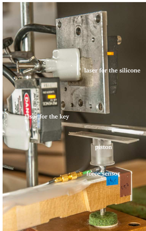
Figure 3.3 – Set-up for actuating the key.
