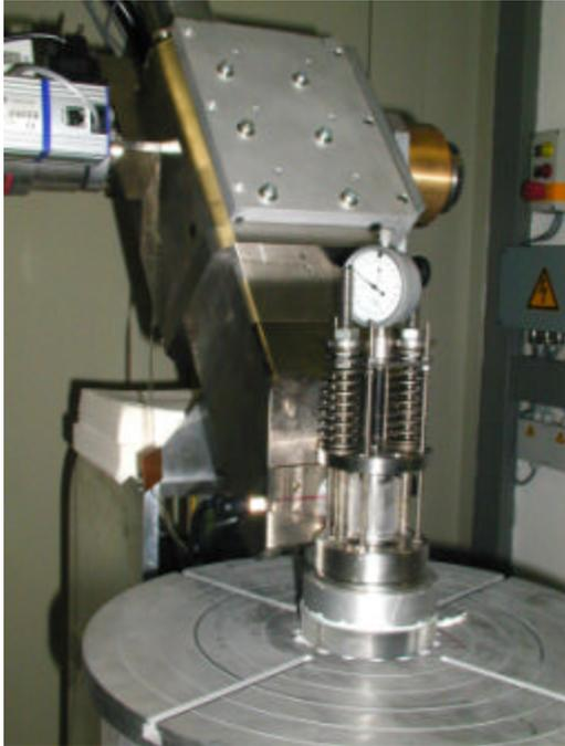
Figure 67: Sample holding device during a solution test under load in front of the X-ray  $\mu$ -focus source with a mechanical  $\mu$ -meter gauge to measure the strain.
