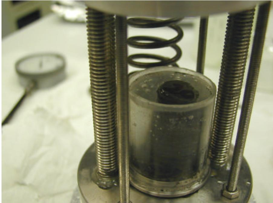
Figure 70: Decharged device with a full reservoir (salt solution) and the specimen in the centre after the test.
