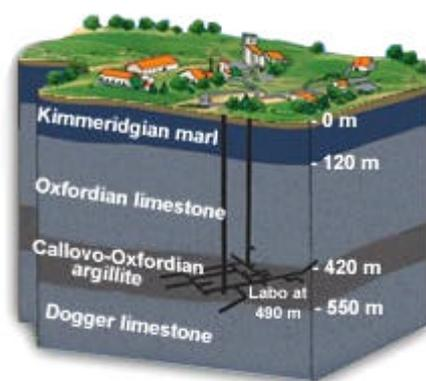
Figure 60: geological 3D model of the underground lab of ANDRA at Bure (ANDRA 2000).
