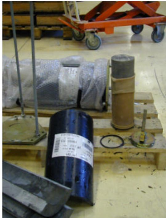
Figures 58 a), b), c), d): Preservation technology used by ANDRA. The specimen is wrapped in a plastic jacket, which is embedded in a casing of concrete. The concrete is moulded in a PVC tube around the core. In the axial direction the sample is charged by a linear compression spring.
