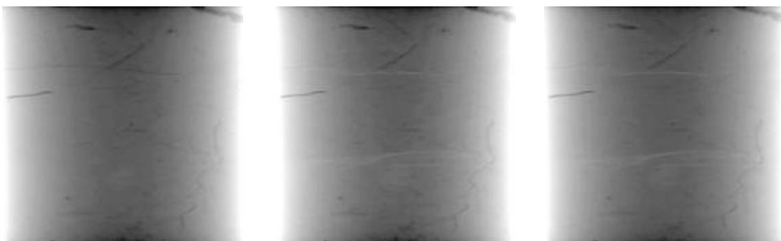
Series 4: specimen #26 in a 1,3 molar KCl solution, immediately after the filling, after 16 minutes and after 40 minutes. Horizontal main crack systems are visible, as well as a few smaller cracks above the upper main crack. Load =1.5 Mpa, T =25°C, picture width = 16mm,  $\mu\text{CR}=22\mu\text{m}$ .
