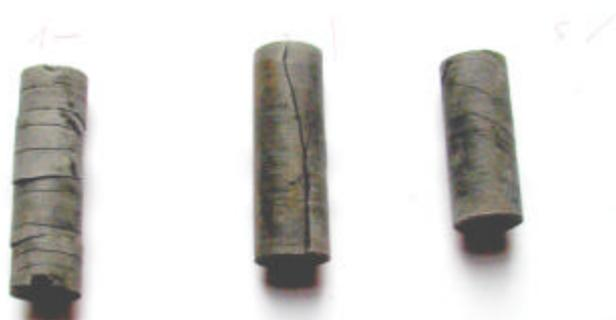
Figure 75: from left to right: specimen #1, #3 and #5, after immersion in a 2 molar KCl solution. The cracks in all three cases are in the direction of the bedding plane:  $90^\circ$  for #1,  $0^\circ$  for #3 and  $45^\circ$  for #5.
