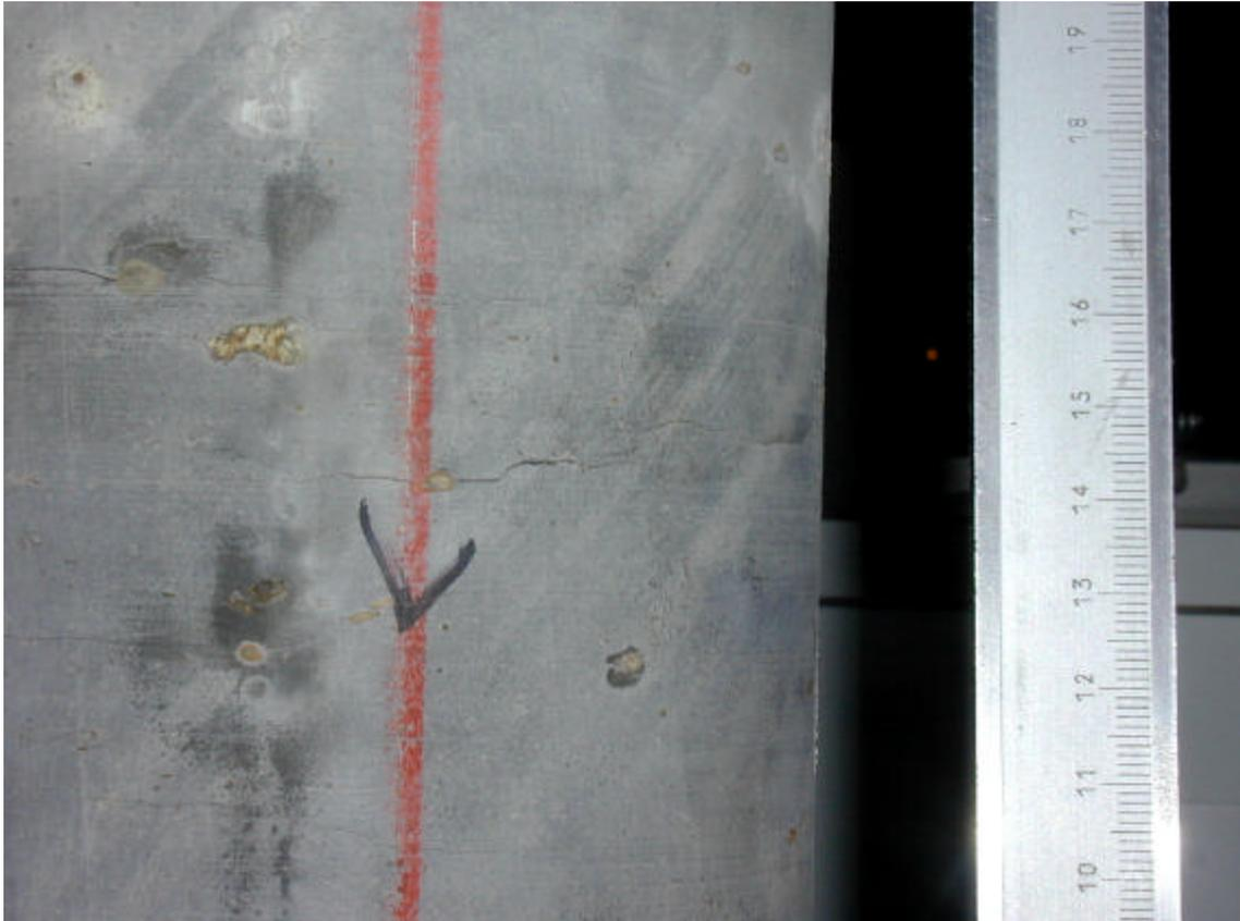
Figure 64: the core sample # 02517 from well 104 immediately after opening the storage device with radially propagated macroscopically visible cracks on the surface – most probably due to dehydration. The inhomogeneities are clearly visible. The colour could also be interpreted as an indication of dehydration
