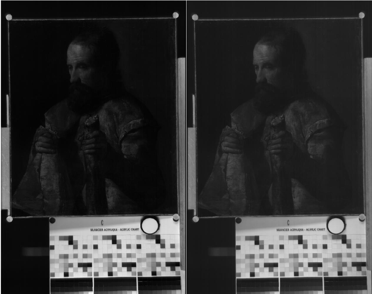
*Figure 8-4. (Left panel) calibrated and corrected image of a Georges de la Tour “Saint Jacques le mineur” painting, (right panel)calibrated but non corrected version.*
