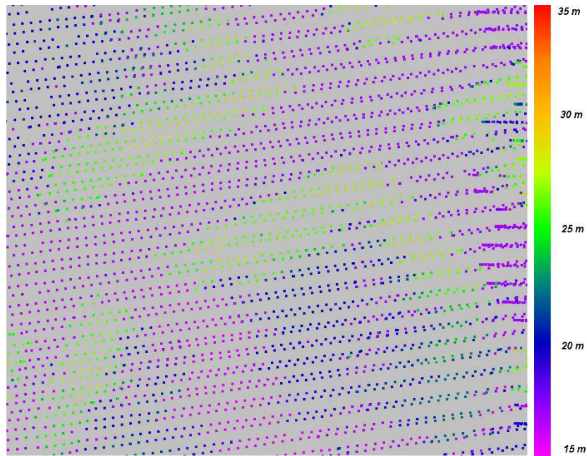
Figure 4.5: Laser scanning points, colors represent altitude values (green points are on the roofs, blue - on the ground).
