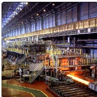
**Roughing mill:** One stand of width reduction is placed after the descaling. Indeed the continuous casting cannot change each time its mould to answer the schedule conditions. Slab width must be sometimes altered. This is performed by a stand with vertical rolls.
