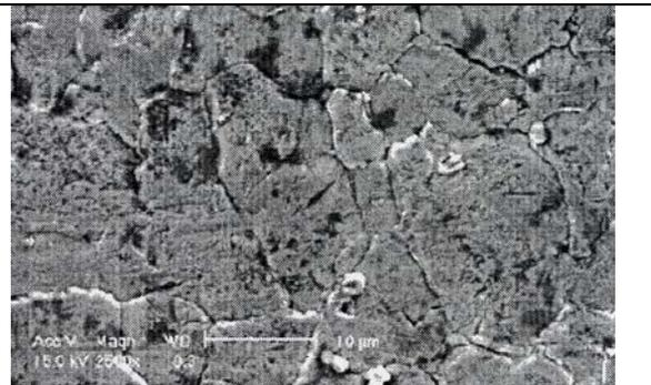
**Figure IV-20: Oxide scale granular morphology: Micrograph of specimen oxidized in air at 900°C and deformed at 800°C [Mou1].**
