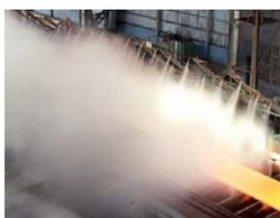
In the finishing mill the product can be sprinkled between each stand, depending on the desired metallurgical treatment.
